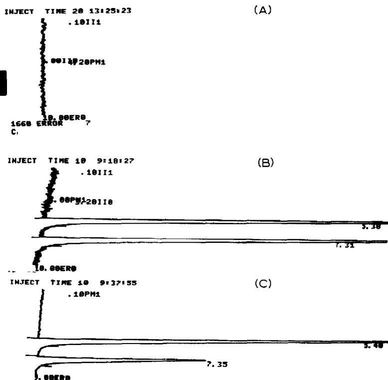
Fig. 1. Chromatograms of (A) a blank plasma sample, (B) a plasma sample spiked with 500 ng of MET per ml of plasma and 500 ng of PRZ per ml of plasma, and (C) a plasma sample of a healthy volunteer, taken 4 h after oral administration of 5 mg of MET.
